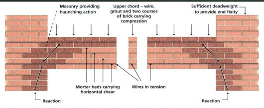
The upper tendon combines with the two surrounding brick courses to enhance compression and the bottom tendon acts in tension to significantly increase the tensile and flexural capacity of the masonry.
